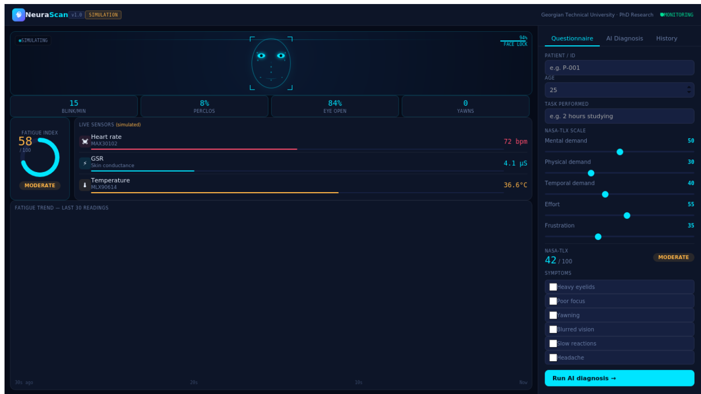
Fig. 1. NeuraScan demonstration interface (simulated data), showing the live eye-tracking overlay with blink rate and PERCLOS, simulated ECG/GSR/temperature sensor readouts, the fused fatigue index ring, and the NASA-TLX questionnaire panel.
